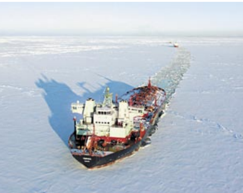
The oil tanker Tempera , 106,000 tons, designed for sailing in ice as well as on open seas. It was the only oil tanker that could sail without the assistance of ice-breakers in the Baltic during the winter of 2003 when the ice was 80 cm thick.
